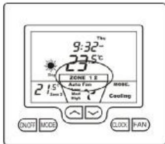
If zoning is enabled the word “Zone” and either “1”, “2,” or “1 2” (indicating both zones) will be shown. To select which zone(s) you wish to be controlled, simply tap the On/Off button to toggle between zone 1, Zone 2 or both zones
