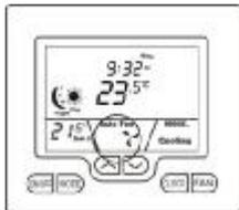
If your air conditioning system has only one Indoor fan speed, the words “High”, “Med” or “Low” will be absent from the TZT-701 Wall Control display, as shown in the picture to the left.
