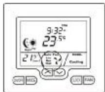
If your air conditioning system has 3 fan speeds, the TZT-701 thermostat will indicate each fan speed in the position shown in the picture to the left.
